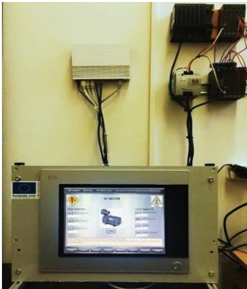
HIL working place based on PLC for control methods verification of drive system
