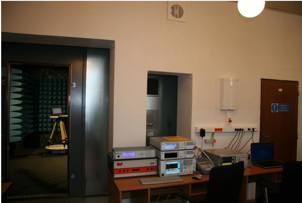
Measuring equipment with un-echoing chamber
