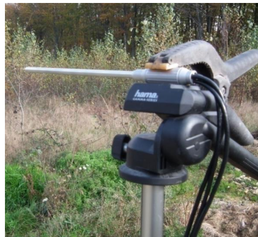
Gauss/Teslameter Model 8030 (on the left) with external sensor (on the right)
