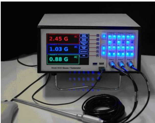
Gauss/Teslameter Model 8030 (on the left) with external sensor (on the right)
